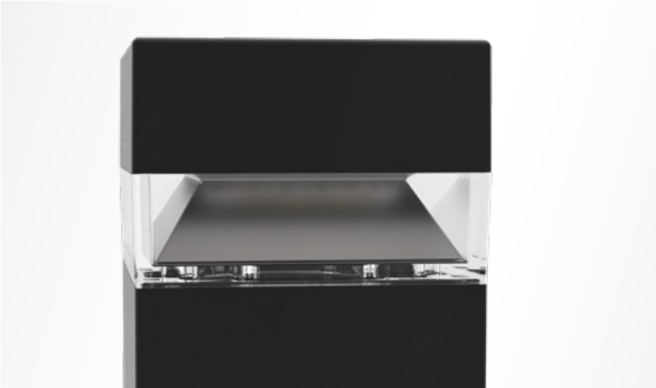
Internal specular reflector coated with 5-layers of PVD 99.98% pure aluminum providing >95% reflection.
