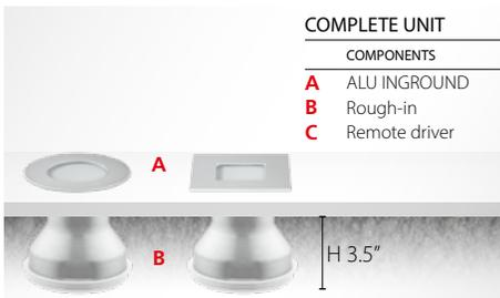
Recessed inground products consist of three parts (codes) to order a complete fixture.
