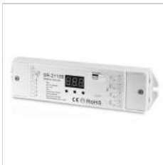
178973 RGBW DMX enabler/decoder 4 channel (0.35A each CH)
