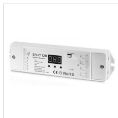
178973 RGB DMX enabler/decoder 4 channel (0.35A each CH)
