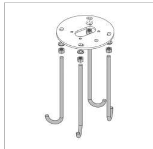
Anchor Bolts w/ template
