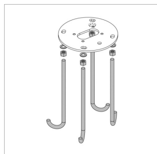
Anchor Bolts w/ template
