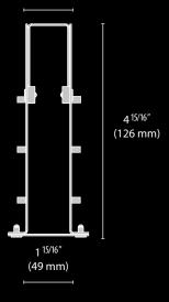
Two-part fitting, consisting of LED luminaire and stainless steel recess box with anti-deformation cover (included). Tool-free installation of the luminaire in the recess box
